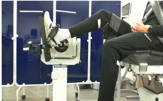
Figure 3.6: Isokinetic dynamometer set up for ankle exercise.
