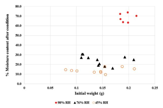
Figure 2. Moisture profiles of post tanned chromium leathers pre-conditioned at 98%, 76% and 45% relative humidity in constant environment chambers. Drying was performed at 23°C.
