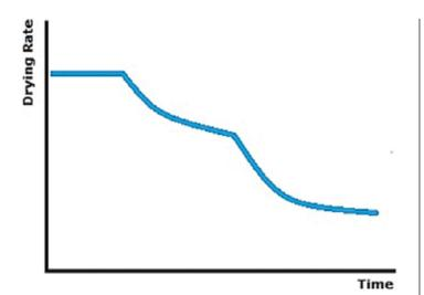
Figure 1. Starting with constant rate drying, the curve moves into the first variable rate drying sequence that is lower than the first phase of drying. A slower third phase of drying shows a marked tailing of the drying rate that is often attributed to removal of bound water. <sup>16</sup>
