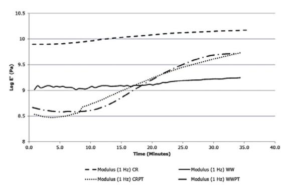
Figure 4. Four damp leather types dried at 60°C in a DMTA instrument and their storage modulus measured at 1 Hz showing variable change in modulus. The leathers were dried where the relative humidity began at 85% and decreased to 45% at 10%/min. The starting moisture content for all leathers was 65% and the post tanned leathers dried to below 10% moisture after 40 minutes.
