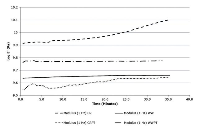
Figure 3. Four damp leather types dried at 40°C in a DMTA instrument and their storage modulus measured at 1 Hz showing variable change in modulus. The leathers were dried where the relative humidity began at 85% and decreased to 45% at 10%/min. The starting moisture content for all leathers was 65% and did not go past 35% in any of the leathers after 40 minutes.
