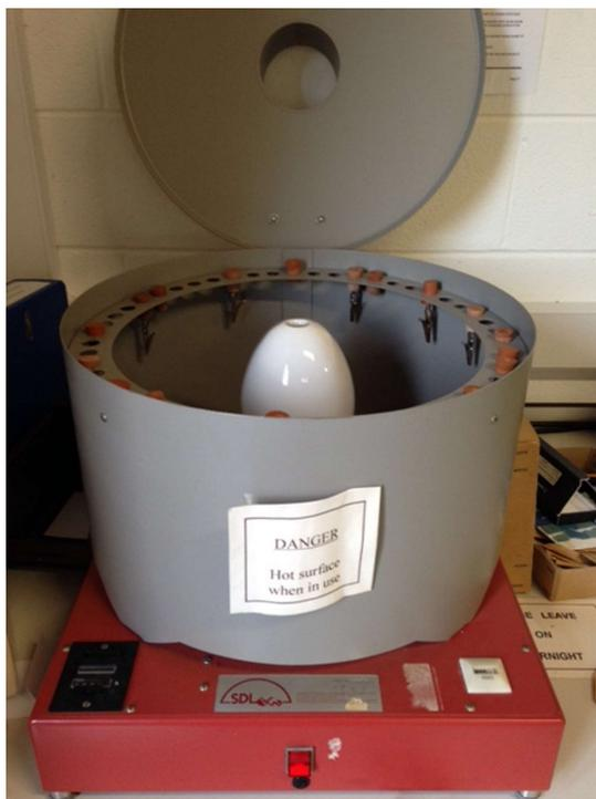
**Figure 3-3:** Chamber for light stability test.
