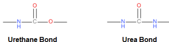
Figure 4–1: The chemical configuration of urethane and urea bonds. The cyanate functional group will form a urethane bonds in reaction with hydroxyl functional groups and urea bond in reaction with amine groups.
