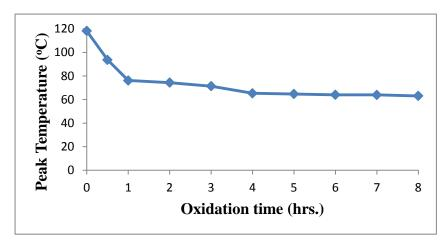
Figure 1: Different oxidation time (hr.) with peak temperature
