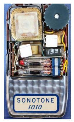
1952: Transistorized consumer products appear and ...... Semiconductors in batterypowered hearing aids and pocket radios.
