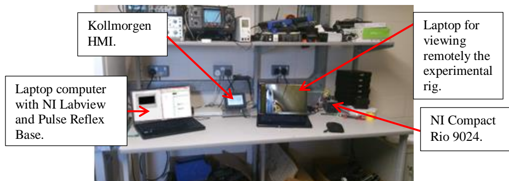
Figure 3.8 Control room for the experimental rig
