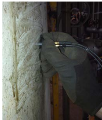
Figure 3. Standard twin crystal normal compression probe at 5 MHz coupled manually to Carbon Steel component.
