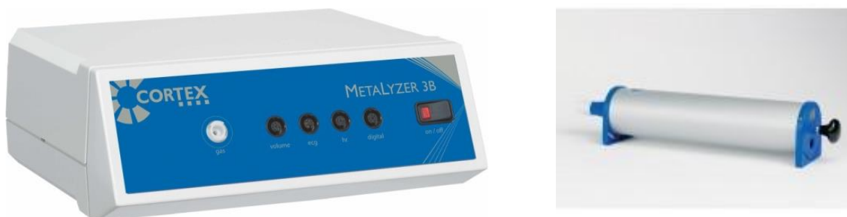
Figure 3.2.2: Cortex Metalyser with accompanying syringe to calibrate flow volume.
