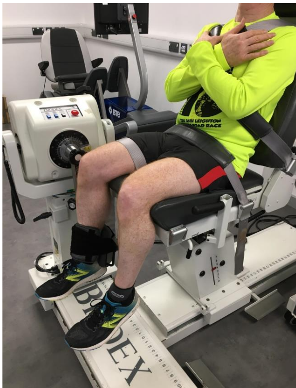
Figure 3.2.1: Standardised positioning of participants on the Biodex Dynamometer.
