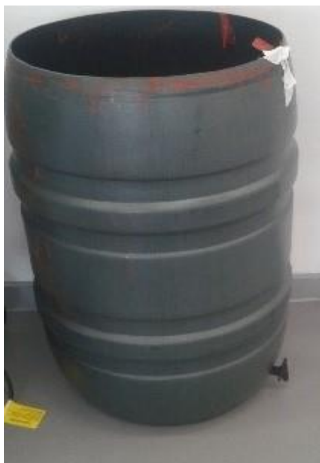
Figure 5.2.1: Plastic water butt used for cold water immersion trials with a total capacity of 200L. Participants were immersed up to waist level in a water temperature of 15°C.
