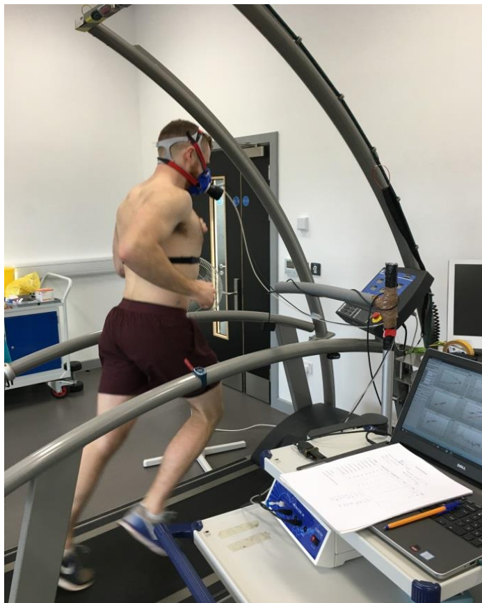
Figure 3.2.3: Participant performing maximal aerobic capacity test to assess VO 2 max. Facemask is linked to Cortex gas analyser.
