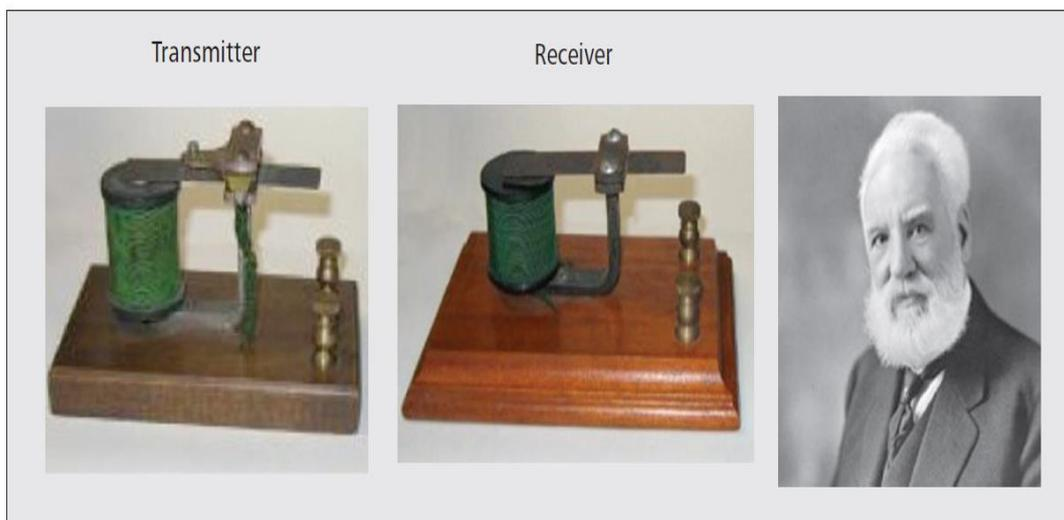
Figure 1.1: Bell's harmonic telegraph system (Schwartz, 2009).
