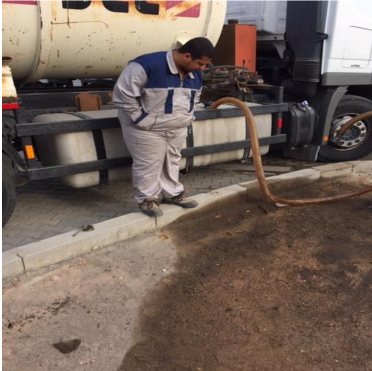
Figure 1.10 - Example of local land contamination due to incorrect handling processes.
