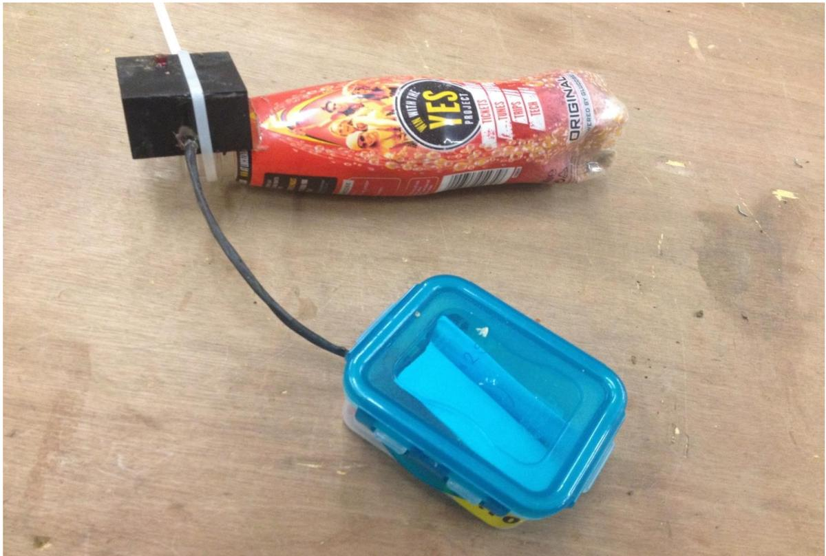
Figure 8.3 - prototype RFID trap. The electronic reader can be seen fitted to the entrance of the bottle and to protect the remaining components these were housed within a waterproof Tupperware box.
