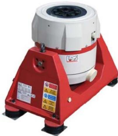
Figure 5-3 Photo of the electromagnetic shaker used in the experiment (Bruel & Kjaer)
