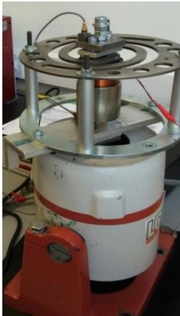
Figure 7-6 Shaker with absorber and VCM test rig
