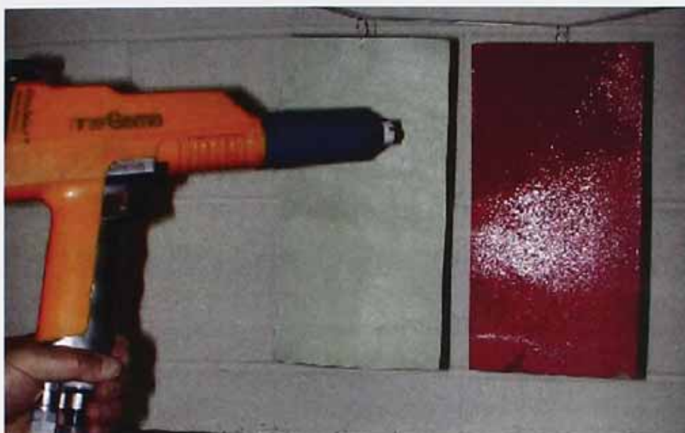
Figure 2.3 Electrostatic spray gun system used
