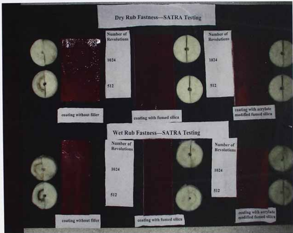
Figure 4.15 Rub Fastness—SATRA testing results of powder coating finished leather
