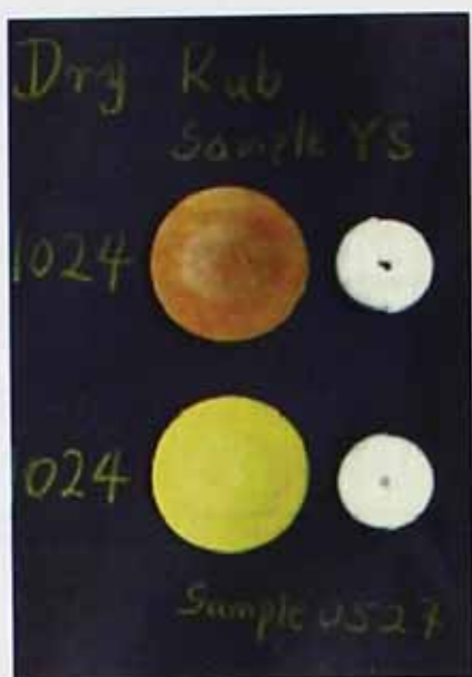
Figure 4.38 Dry rub fastness samples of UVPC-1 and UVPC-2 (the number of rotations of the pad are indicated on the left of the figure)
