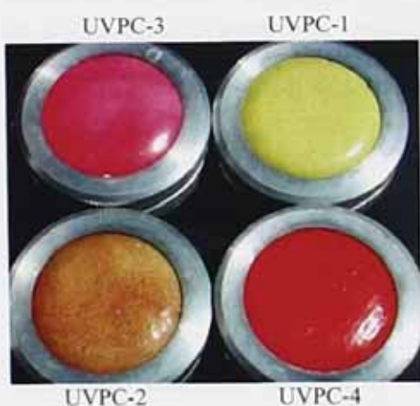
Figure 4.40 Appearance of Martindale abrasion test samples before testing: formulations UVPC-1, UVPC-2, UVPC-3 and UVPC-4
