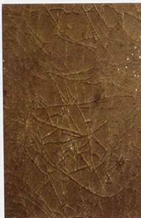
Figure 4.33 A leather sample finished with a powder coating based on Rucote® 7008 resin showing cracking after bending.
