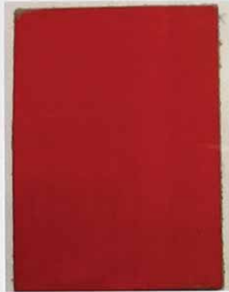
Figure 4.9 Red powder coating finished leather without pre-fusion, hot plating at 100°C
