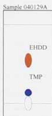
Figure 3.8 TLC method used for monitoring the synthesis and purification processes used during preparation of monomer
