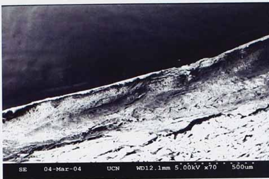
Figure 4.35 An SEM image of a leather sample finished with a powder coating based on the mixture of Uvecoat™ 3003 and Uvecoat™ 9010 resins applied by the EMB finishing method
