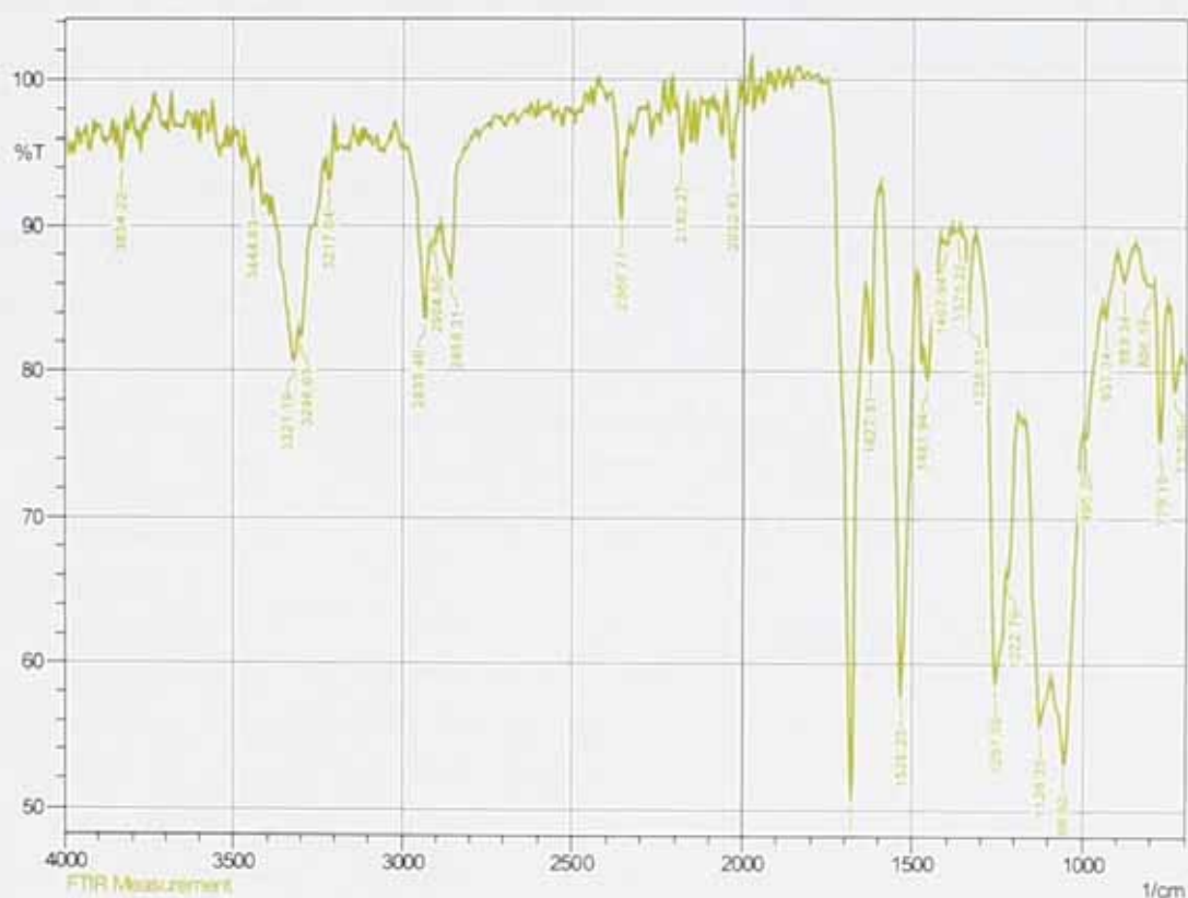
Figure 3.16 FTIR- ATR spectroscopy of polyurethane sample PU-6
