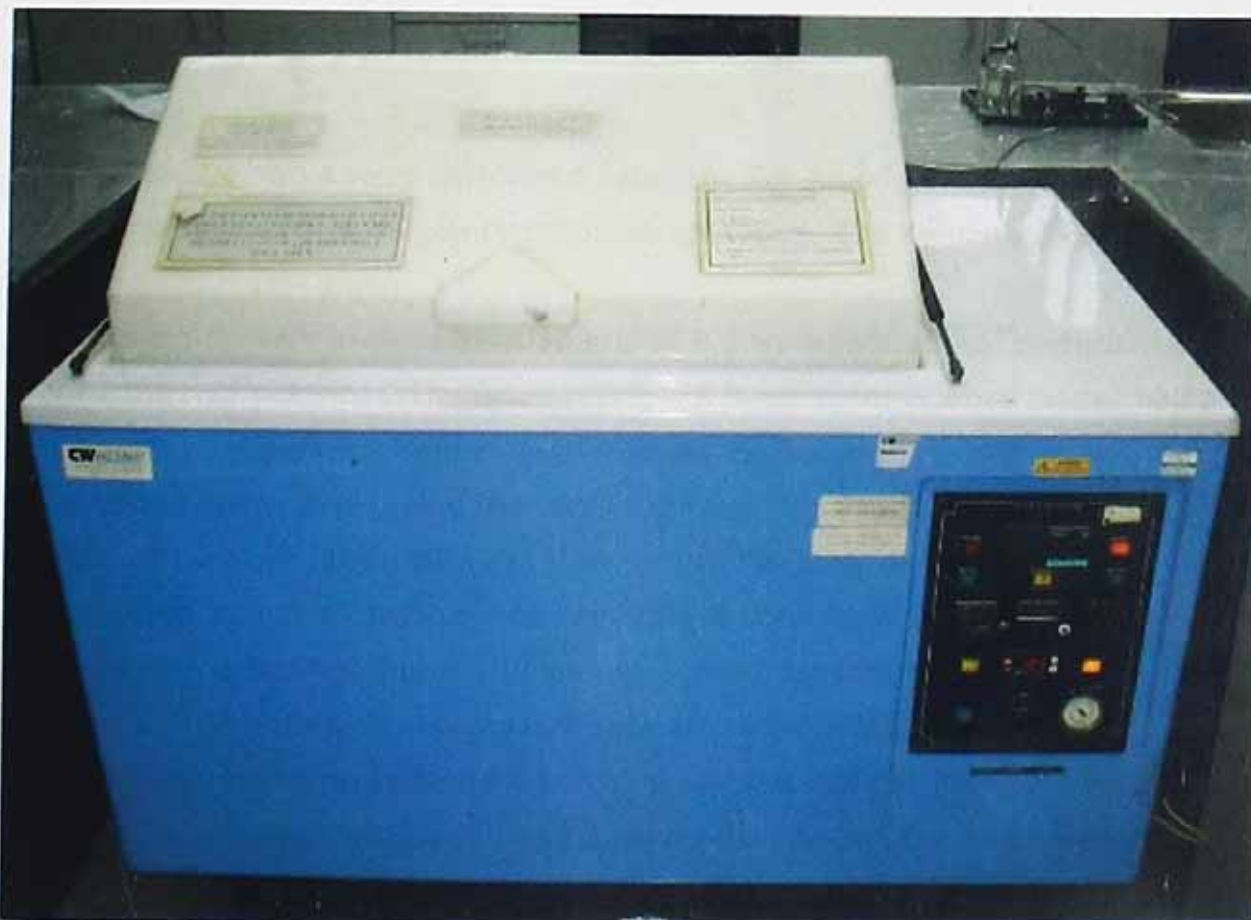
Figure 1 Accelerated weathering cabinet for both Prohesion testing and continuous salt fog exposure (ASTM B117)
