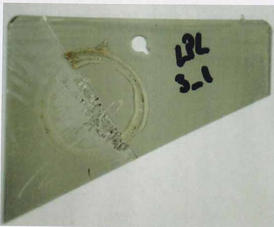
Figure 43. Paint LPL3 after 2500hrs immersion – coating partially removed to show a small area of the underlying substrate
