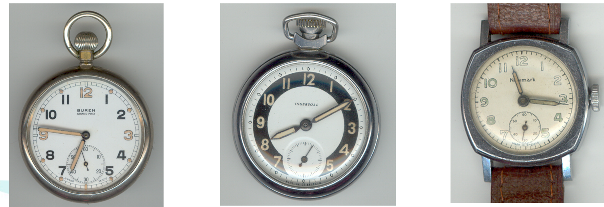
Fig 1. Typical Radium-Dial Watches Left: Buren pocket watch, Swiss, 1940s Centre: Ingersoll pocket watch, UK, 1930s-1950s Right: Newmark wrist watch, UK, 1960s
